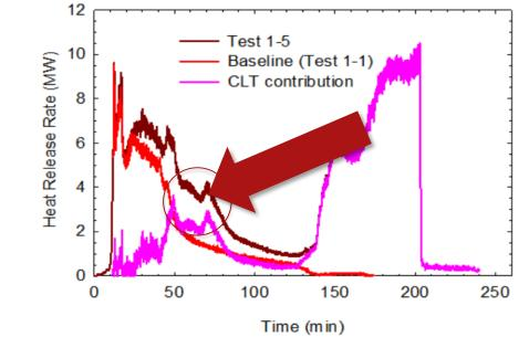
Figure 89. CLT contribution to heat release rate in Test 1-5 (baseline time shifted).
