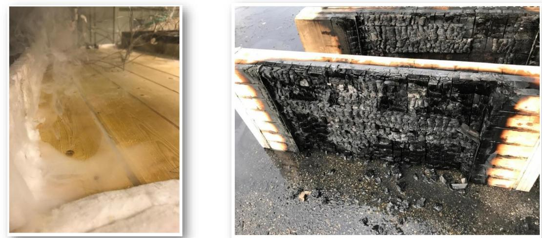
Delamination of Cross-laminated timber and its impact on fire development Focusing on different types of adhesives, Eric Johansson, Anton Svenningsson - 2018
