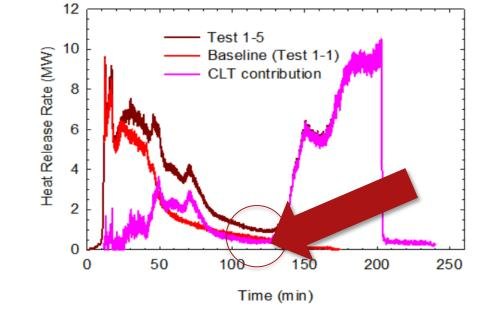
Figure 89. CLT contribution to heat release rate in Test 1-5 (baseline time shifted).
